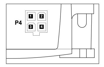
Figure 1.2.4: P4 — 4-Pin Locking Wire Crimp Pin Configuration
